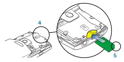
Replace the A cover: insert the two catches on the sides of the cover into the corresponding slots in the phone and slide the cover until it locks in place.
