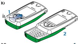
Open the A-cover: with the back of the phone facing you, put your thumb in the middle of the cover, slide it forward and then lift it.
